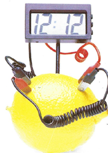
Figure 8 This cell uses the juice of a lemon as an electrolyte and uses strips of zinc and copper as electrodes.
